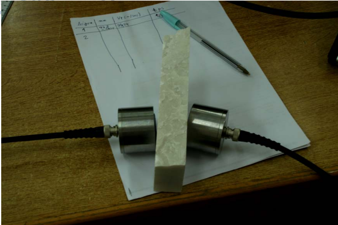
Σχ. 4.4. Ultrasonic Test Equipment - Pundit Lab της proceq.
