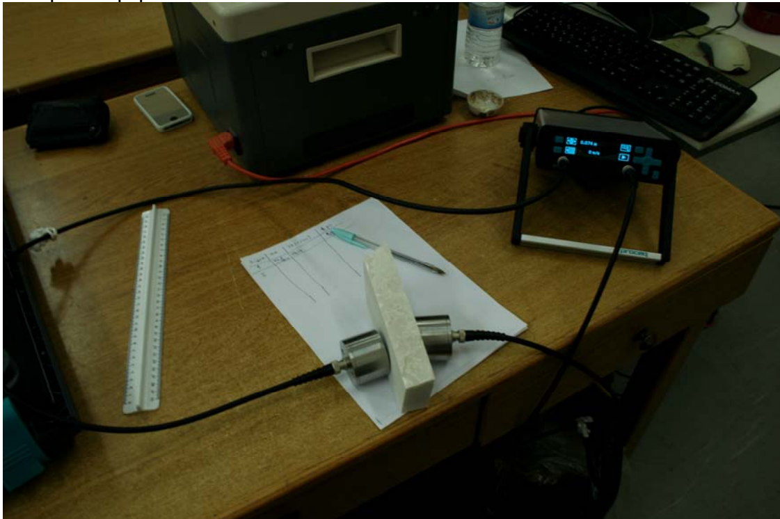
Σχ. 4.3. Ultrasonic Test Equipment - Pundit Lab της proceq.
