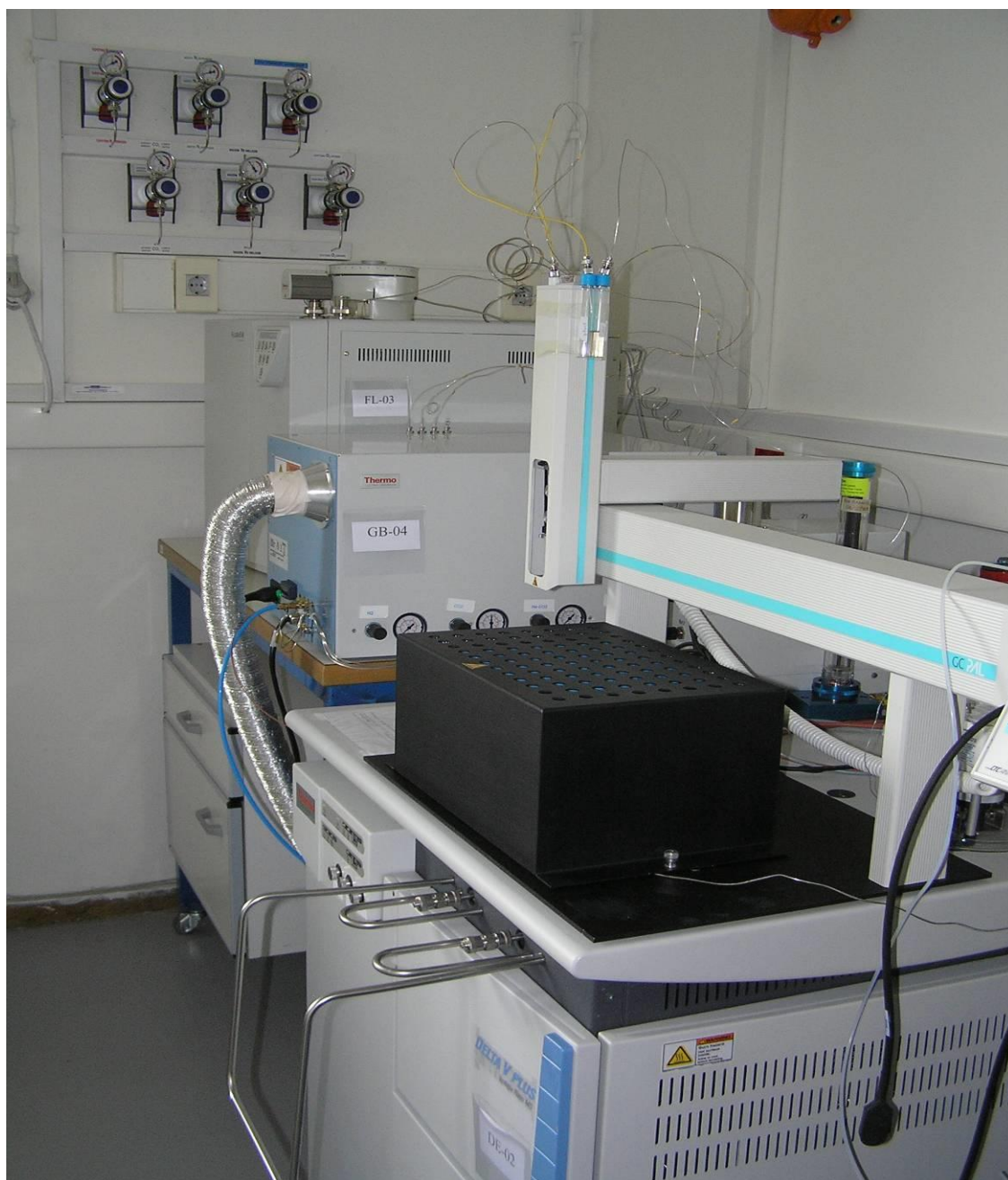
Σχήμα 4.2.6: DELTA V Plus, ThermoScientific, Isotope Ratio Mass Spectrometer
