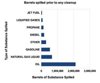
Hazardous Liquids Spilled from Pipeline Incidents 1986 - 2013
