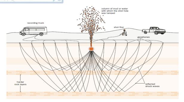
Figure 3.2.1.1: Geophysical surveys in the imminent area at the stage of exploration (Source: UNEP, 1997).
