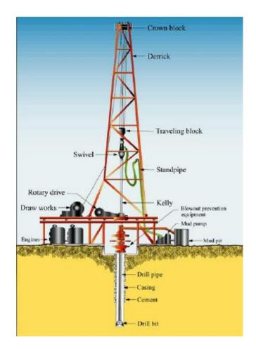
Figure 2.2.1: The form of an onshore drilling rig (Source: https://www.researchgate.net).
