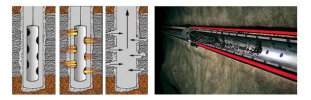
Figure 3.2.2.1: Well completion with the method of perforation, a drilling technique for the oil extraction (*Source: Stamataki*, 2017).
