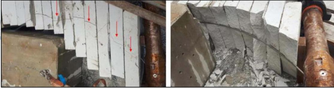
**Figure 9:** Needle deployment verification test regarding the method of multilateral jetting stimulation technology. Foamed cement blocks were used as substitute for the reactive rock. (Bjørnseth et al., 2019)
