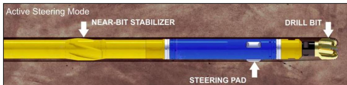
**Figure 19:** Part of a push-the-bit rotary steerable system assembly. (Hakam et al., 2014)
