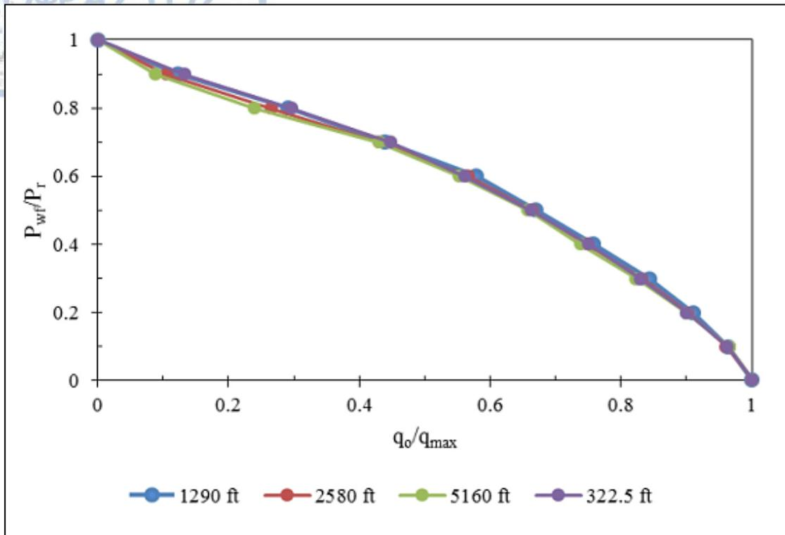
**Figure 34:** Comparison of dimensionless IPRs for various distances between the laterals. (Abdulazeem & Alnuaim, 2016)
