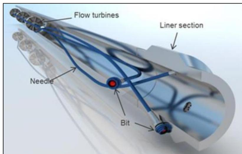
**Figure 12:** The internal structure of a multilateral drilling stimulation technology sub that houses a small-diameter drill bit at the end of each of the three needles. Small turbines inside the liner are connected to the needles and their rotation during the circulation of a high-pressure fluid provides the necessary torque to the bits. (Rice et al., 2015)
