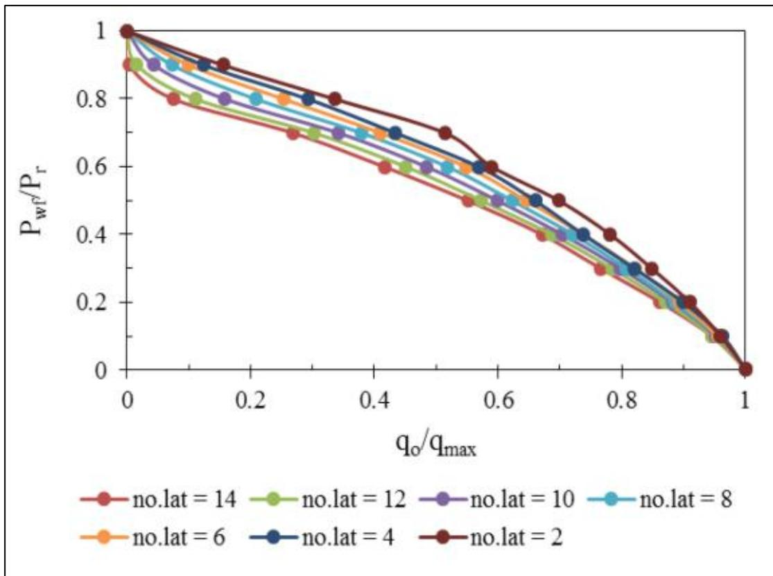
**Figure 24:** Comparison of dimensionless IPRs of fishbone well in relation to the number of laterals. (Abdulazeem & Alnuaim, 2016)
