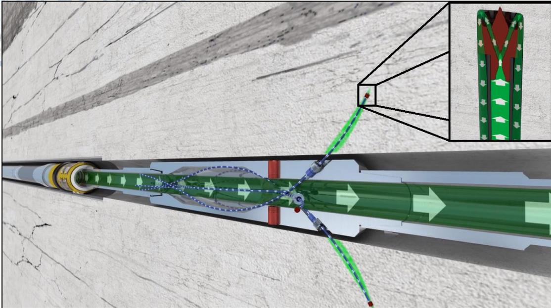
**Figure 8:** Schematic illustration of the jetting process during the extension of the drilling needles regarding the method of multilateral jetting stimulation technology. The arrows indicate the direction in which the hydrochloric acid is moving as it is forcibly pumped into the liner. As it exits the needles, it corrodes the carbonate rock, and due to the pressure exerted on the needles, they penetrate deeper into the rock. (Fishbones AS)
