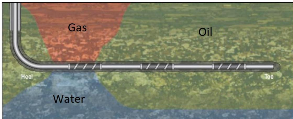
**Figure 30:** Demonstration of the “Heel-to-toe phenomenon that causes water and gas coning due to the greater drawdown pressure at the heel of a long horizontal well, which in turn causes higher inflow at the heel compared to that at the toe. (Manish et al., 2015)
