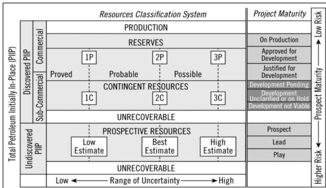
**Figure 1:** The hydrocarbon resources classification system of Petroleum Resources Management System, published by the Society of Petroleum Engineers Oil and Gas Reserves Committee. (Canbaz et al., 2020)
