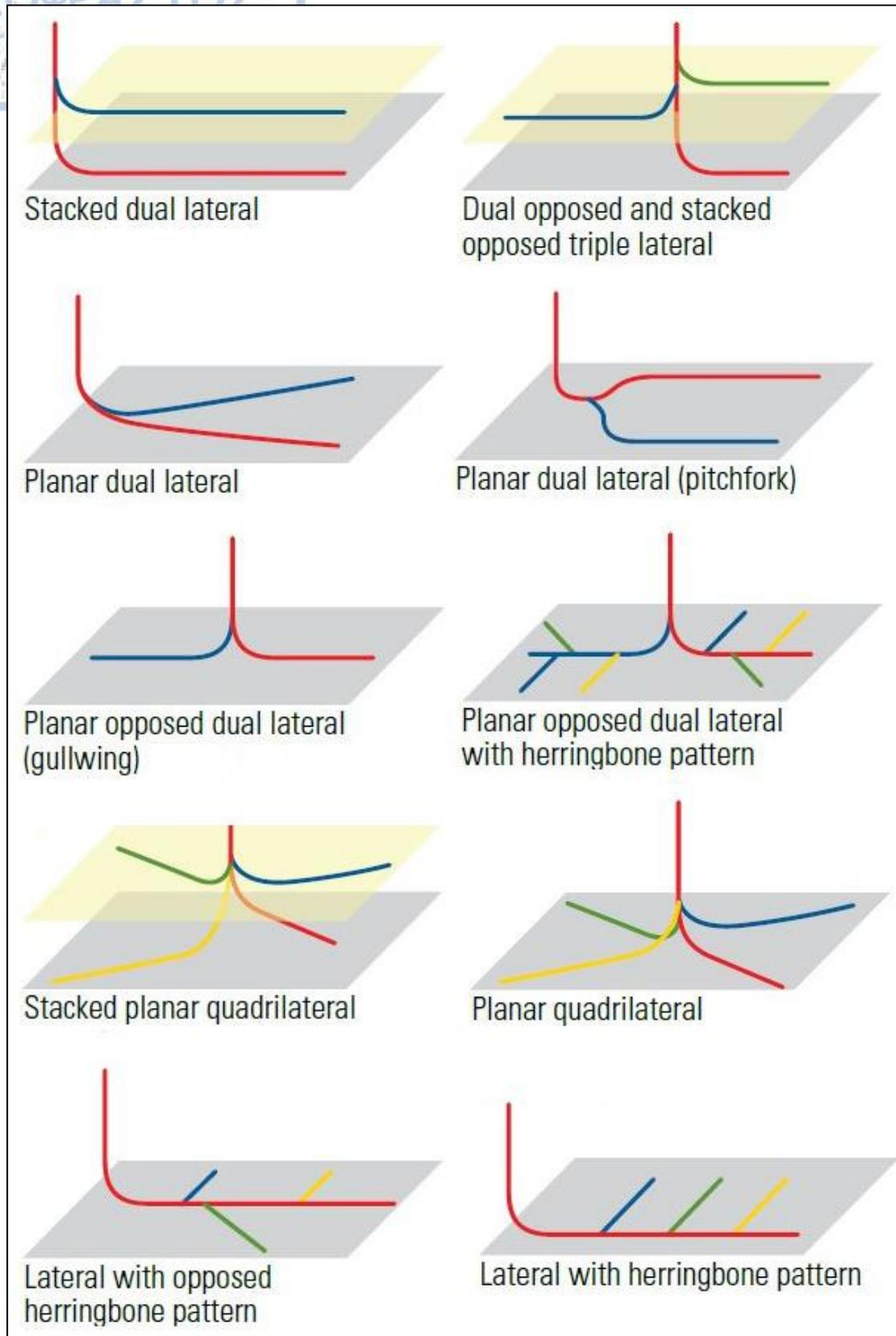
**Figure 3:** Schematic representation of the various types of multilateral wells.
