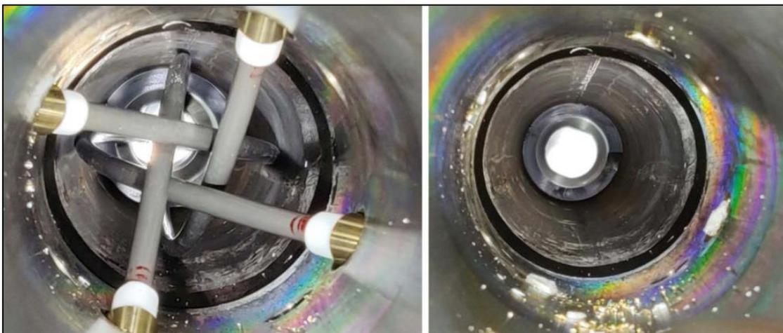
**Figure 10:** Multilateral jetting stimulation technology sub hosting four needles.
