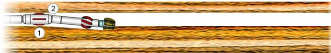
**Figure 20:** Representation of the sidetracking sequence at the kick-off point performed by a point-the-bit rotary steerable system. The procedure begins with the ledge building phase. The bias unit is in close contact with the walls of the main horizontal well (1) and the drill bit is pointed downwards with the maximum possible deflection (2). (Voronin et al., 2017)
