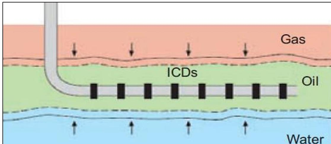
**Figure 31:** Prevention of early inflow of unwanted fluids using Inflow Control Devices that balance the inflow along the entire length of a horizontal well. (Manish et al., 2015)
