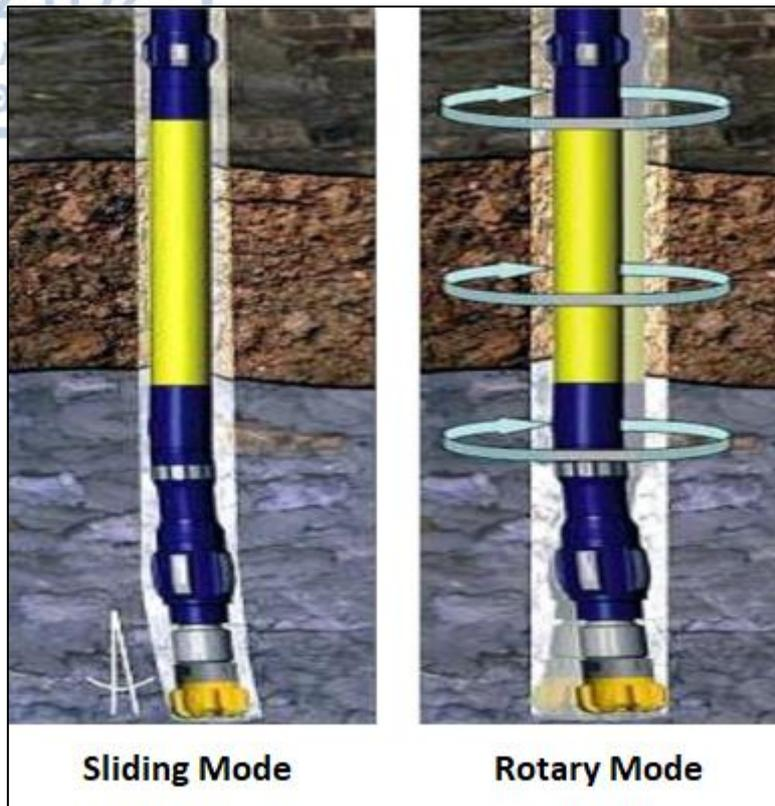
**Figure 16:** Representation of a mud motor assembly in sliding and rotary modes. During the rotary operation where the entire drill string rotates, an interval of larger diameter than normal is drilled. (Al Dabyah et al., 2016)
