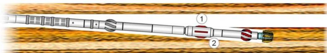
**Figure 21:** The "time drilling" phase of the sidetracking sequence, the objective of which is to build a tangent section that is long enough to host the bottom hole assembly. The process begins with the ledge building phase. The interval of an enlarged hole in which the bias unit must operate makes any guidance of the bit impossible (1). Thus, the tangent section is drilled with the bit in the neutral position (2). (Voronin et al., 2017)
