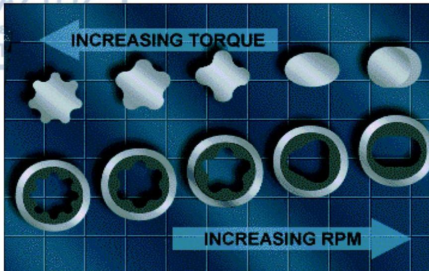
**Figure 15:** Various configurations of a rotor – stator system. The number of lobes determines the torque of the system and the rotational speed of the rotor. ([https://petrowiki.spe.org/Directional\\_deviation\\_tools](https://petrowiki.spe.org/Directional_deviation_tools))
