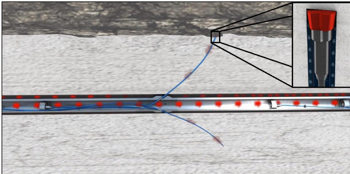
**Figure 13:** Representation of the drilling phase regarding the method of multilateral drilling stimulation technology. The arrows indicate the flow of drilling mud, through which the cuttings powder is circulated to the surface. (Fishbones AS)
