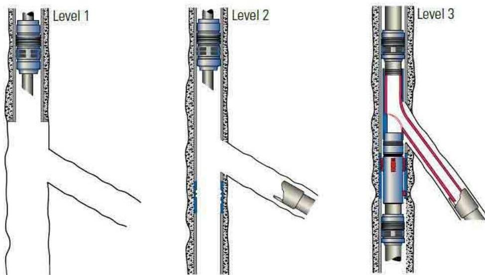
**Figure 4:** Schematic illustration of levels 1, 2, and 3 of the TAML classification system.
