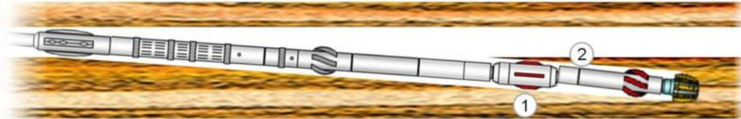
**Figure 22:** The “ramp-up” phase of the sidetracking sequence, the objective of which is to further separate the two boreholes. Since the bottom hole assembly is inside the tangent section, the bias unit has regained contact with the walls so the drillers can re-direct the drill bit (1). From then on, adjustments are made to the bit’s inclination and azimuth to continue drilling the lateral in the desired direction (2). (Voronin et al., 2017)
