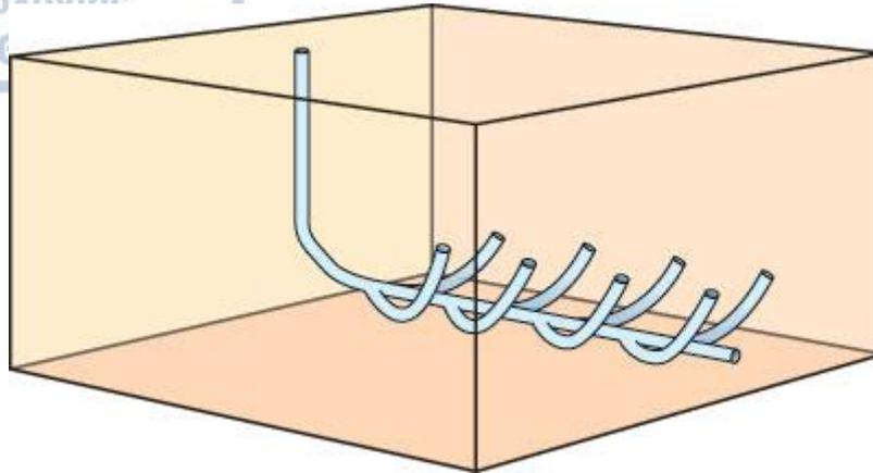
**Figure 6:** Schematic representation of a fishbone well.
