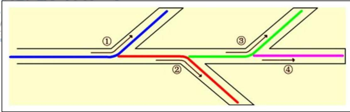
**Figure 14:** Schematic representation of the forward drilling method where every new lateral is a sidetrack of the previous one. Part of the main wellbore and the first lateral are drilled first (1), followed by a kick-off operation to drill the next part of the main hole along with the second lateral (2). The same process gets repeated for the third lateral (3) and finally the last part of the main well is drilled (4), which is a sidetrack from the last lateral. (Yu et al., 2012)
