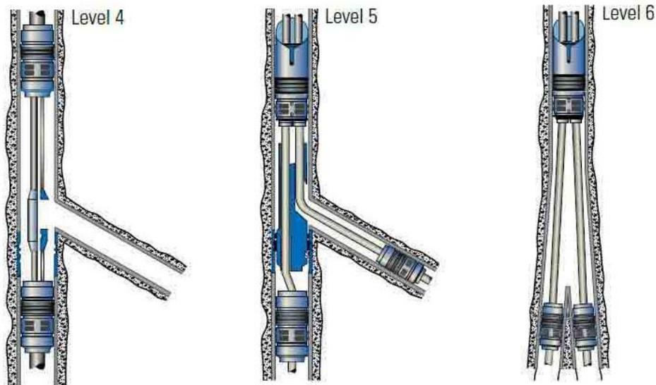
**Figure 5:** Schematic illustration of levels 4, 5, and 6 of the TAML classification system
