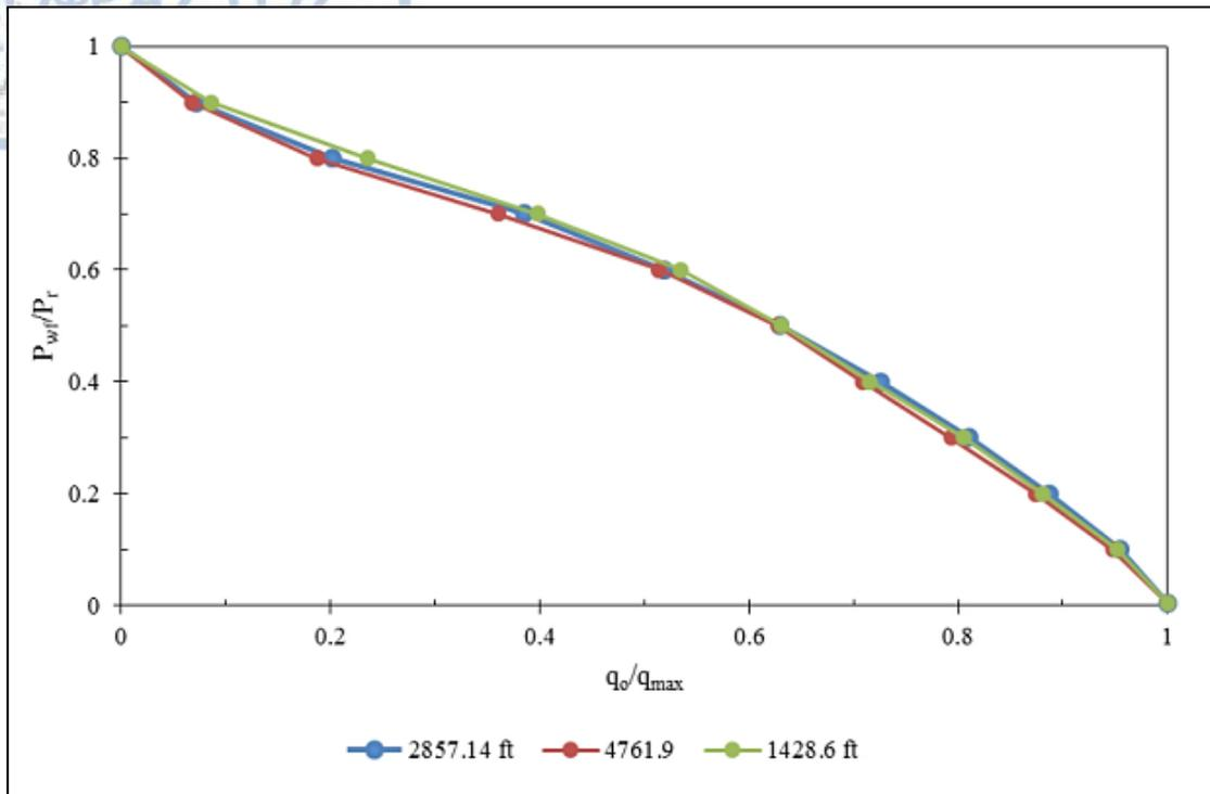
Figure 28: Comparison of dimensionless IPRs for different lengths of laterals. (Abdulazeem & Alnuaim, 2016)
