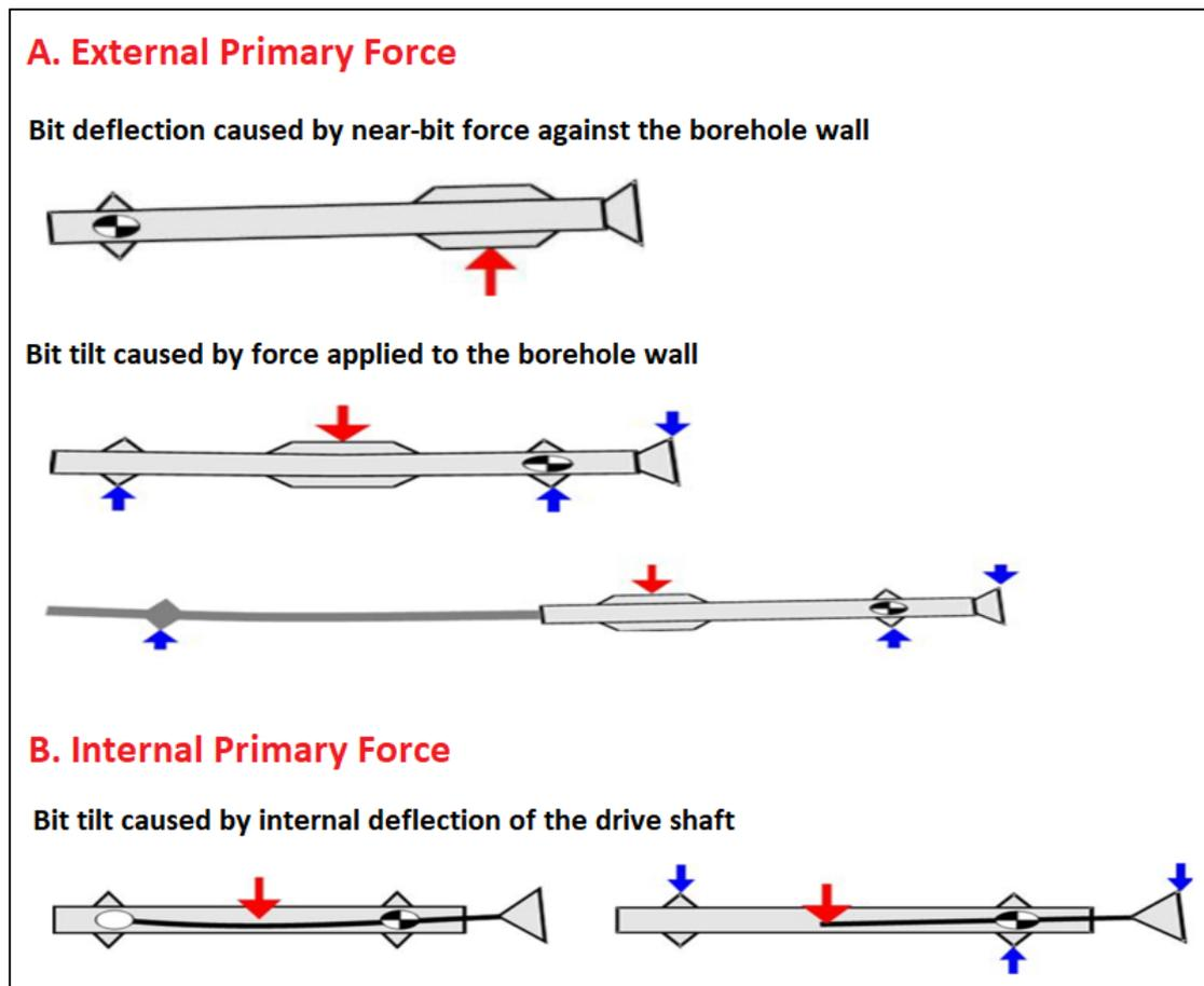
**Figure 17:** Categorization of rotary steerable systems based on the position of the primary force causing the bit deflection. This initial force is symbolized by the red arrows, while the blue ones represent the secondary forces that develop. The circles are the fulcrum points, on either side of which the direction of movement is reversed. (Al Dabayah et al., 2016)
