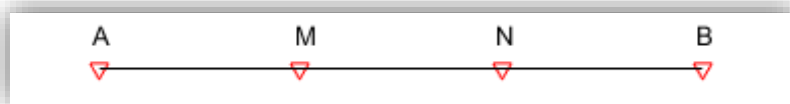
Figure 2.2: Arbitrary arrangement of 2 current electrodes ( A^{(+)} and B^{(-)} ) and two potential electrodes (M and N).
