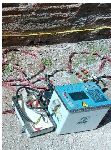
Figure 2.9: The Syscal pro instrument, that was used for the acquisition of the measurements.
