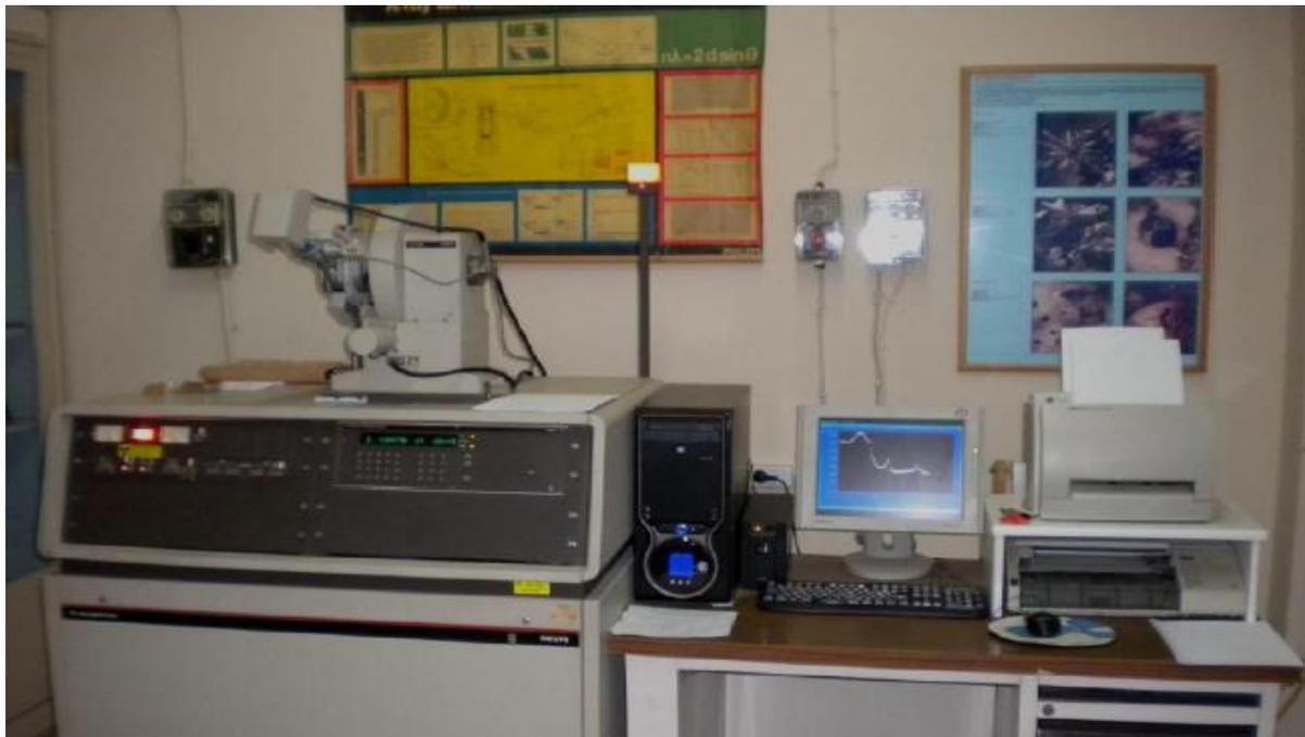
**Figure 5: X-ray diffractometer (XRD), Philips PW1820/00-type, Department of Mineralogy-Petrology-Economic geology, Aristotle University of Thessaloniki.**
