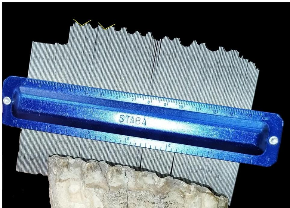
**Figure 4.** Measuring of the mesowear angles with the use of a contour gauge.
