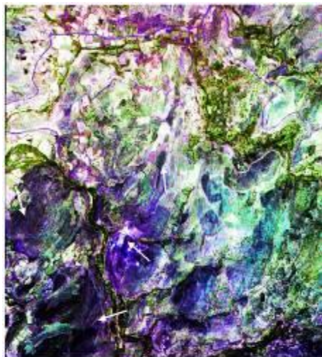
Fig. 4 RGBI display of the first 4 MNF components (3= R, 2=G, 4=B, 1=I). Arrows show marble formations
