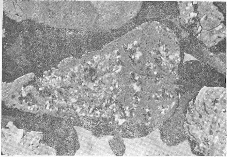
Fig. 17. The same as in fig. 16 under crossed Nicols. Pyrolusite is distinguished due to its strong anisotropy (white parts).
