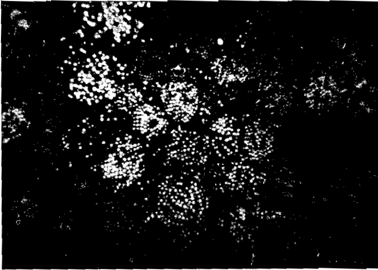
Fig. 3. Framboids with very different shapes (pyrite crystals are white) Polished section. Oil immersion, 1500 X.
