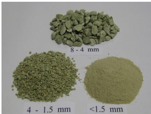
Fig. 2. The grain-sizes of HENAZE (< 1.5 mm used for the batch-type experiments).
