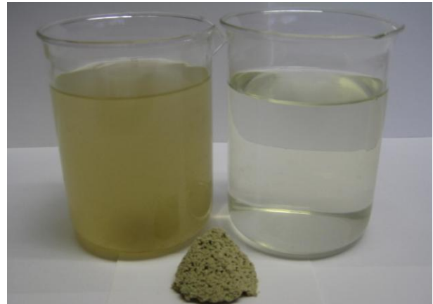
Fig. 3. Left: Starting municipal wastewater, Centre: Odorless and cohesive zeo-sewage sludge, Right: Overflowed clear water.
