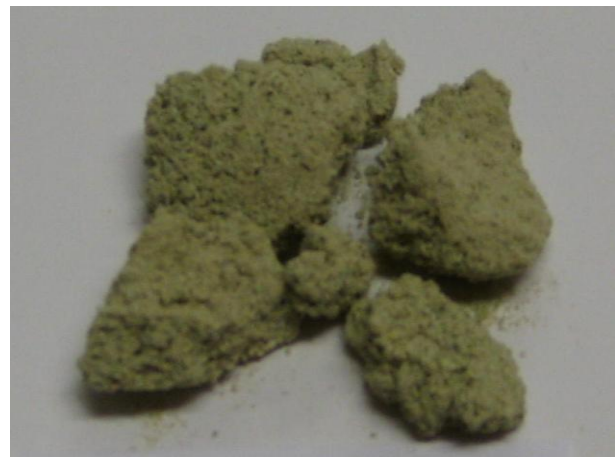
Fig. 4. Odorless and cohesive zeo-sewage sludge, dried overnight at RT.
