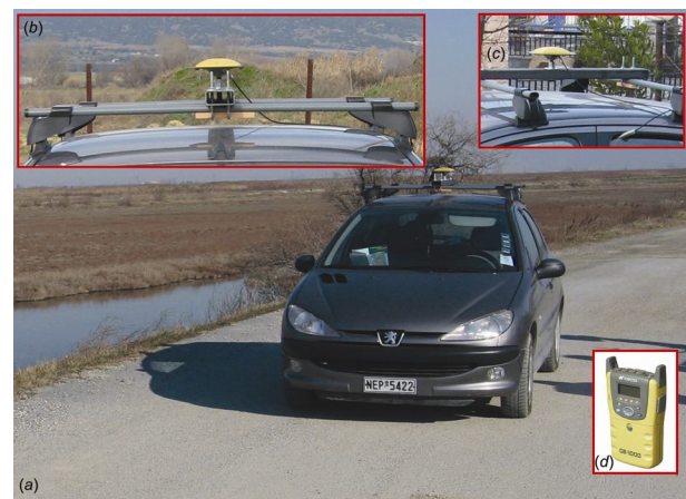
Figure 15. Rover receiver antenna (b, c) mounted on the top of the vehicle (a) that was used during the KGPS measurements. One of the 2 identical Topcon™ GB-1000 receivers that were used is also depicted (d).
